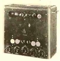
\* Sixty-watt power amplifier using 6L6 beam tubes. Approximately same physical size as old-type 30-watt amplifier. Has one to four position input—gain 143 DB. Tapped output impedance—will handle 1 to 10 permodynamic speakers. Amplifier will serve from 12-12,000 people, depending upon conditions. Model 4P-60. Webster-Chicago, 3825 W. Lake St., Chicago, Ill.—Radio Today—see also advt. p. 31.
