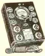
★ Tube tester for metal, "G" and glass tubes. Leakage tests up six megs. D'Arsonval English reading meter. Rotary switch for testing each element of tube. Filament rotary switch for all voltages. Checks paper by-pass Condensers and leakage in electrolytics. Steel case — 7 x 10 x 3½. Model EE — net \$18.95. Million Radio & Television Labs., 361 W. Superior St., Chicago, Ill. — Radio Today
