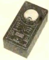
\* Pocket type volt-ohm-milliameter with selector switch and black molded case. DC ranges — 0/15/150/750 volts, 1.5/15/150 mils, ½-1,000, 0/100M ohms with 1.5 volt battery. 2-inch Triplett D'Arsonval meter. Case with rounded corners — 3 1/16 x 5% x 2½ inches. Modernistic silver and black panel. — Model 735 — net \$10.80. Readrite Meter Works, Bluffton, Ohio — Radio Today — see also advt. p. 61.
